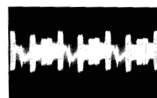
4. IC601 Pin 40 (E-PCB) B-Y In 0.2V, 20 \mu s / Div
