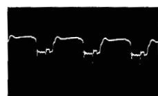
16. Q501 Base (E-PCB) Horizontal Out 18.0V, 20 \mu s / Div
