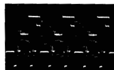
1. IC101 Pin 20 (E-PCB) Composite Video Signal 2.3V, 20 \mu s / Div
