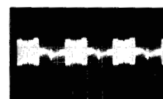
5. IC601 Pin 38 (E-PCB) R-Y In 0.2V, 20 \mu s / Div
