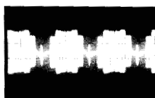
3. IC601 Pin 47 (E-PCB) Chroma In 0.3V, 50 \mu s / Div
