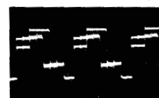
9. E-32 (E-PCB) Green Output From Ic601 Pin 3. 4V, 20 \mu s / Div
